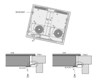
$\underline{M}$  Under any circumstances, the brackets cannot touch with the inner surfaces of the worktop after installation (see picture).
